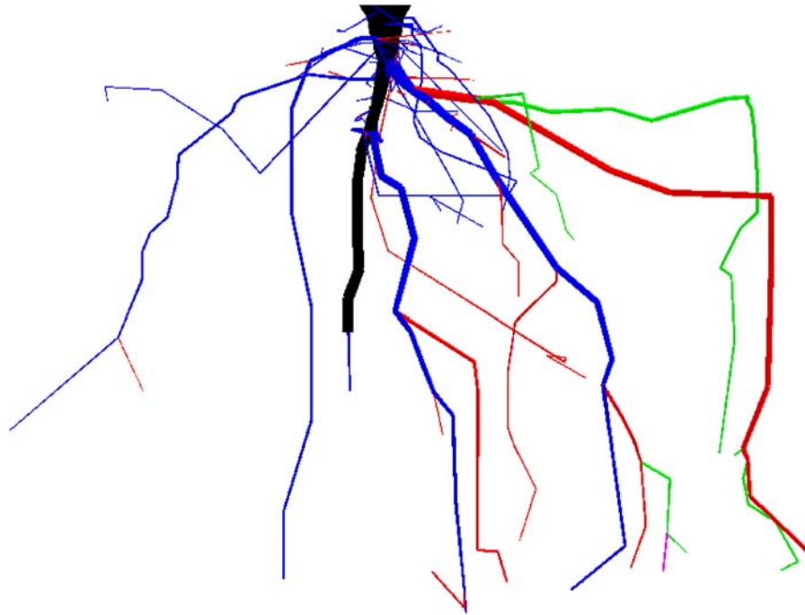
Fig. 1 Graphical reconstruction of a mature Euclea racemosa root system in Tigray (Northern Ethiopia) using the AMAPmod software. Full manual excavation using spade, pickaxe, shovels and spoons, and taking care to maintain all root segments >3 mm in their original position takes about 6 man days. Measurement performed within 2 days using a simple compass,
